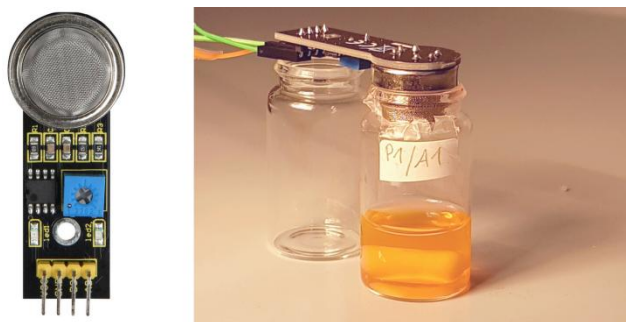
Figure 6. Low-cost hydrogen sensor (left); the sensitivity can be regulated via the potentiometer (colored in blue with gray screw); simplified hydrogen concentration measurement (right)
