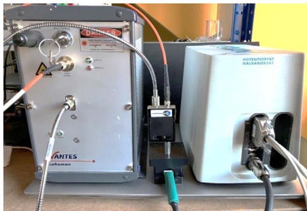
Figure 6. SERS set-up. From left to right: Raman spectrometer with 785 nm laser, Raman probe with Raman cell. Inside the Raman cell: SPE with connection to potentiostat (right). The potentiostat triggers the Raman spectrometer
