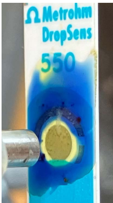
S7. Decolouration of a solution of thymol blue on a Pt electrode after 60 s of electrolysis at 2V.
