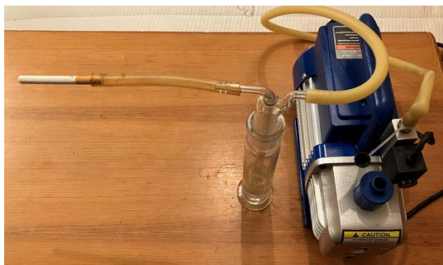
Figure 2. Apparatus for washing cigarette smoke. From left to right: cigarette, bubbler, pump
