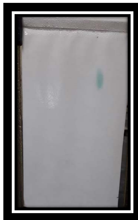
Figure 3. Separation of metal ions ( \text{Ni}^{2+} and \text{Co}^{2+} ) by paper chromatography by using 1% \text{NH}_4\text{OH} solution
