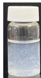
Figure 12. An example of the gel generated from cicada shells after dialysis against 12,000-14,000 Da molecular weight cutoff.
