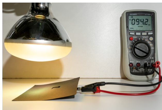
Figure 5. Experimental setup for the comparison between silicon and perovskite solar cells.
