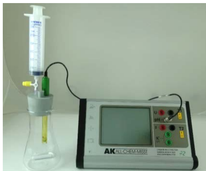
Figure 3. Reactor for biogas production in a school experiment with pH monitoring
