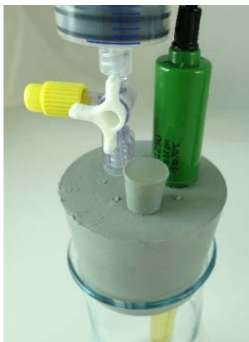
Figure 2. Three-hole stopper at the top of the biogas reactor used in a school experiment
