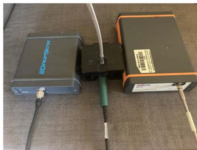
Figure 3. Two used experimental setups. Top: Potentiostat and ECL cell with photodiode. Bottom: Potentiostat with spectrometer and homebuilt cell with lens, fiber and the adapter for SPE.
