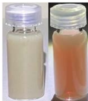
Figure 1. Dichroic colloidal solution of silver nanoparticles in reflected light (left) and transmitted light (right)
