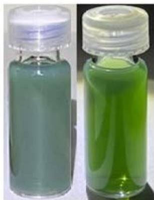
Figure 4. Dichroic colloidal solution of silver nanoparticles formed in the presence of \text{CuSO}_4 in reflected light (left) and transmitted light (right)
