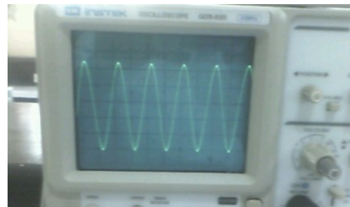
Figure 2. Modulating Signal displayed at Elect./ Compt. Laboratory, LASU
