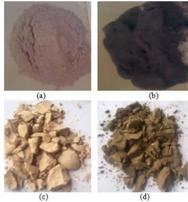
Figure 1. (a) Bentonite powder (b) Olokoro clay (as mined) (c) Dried Olokoro clay (d) Dried Olokoro clay mixed with Bentonite
