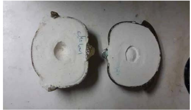
Figure 7. The dewaxed duplicated cast
