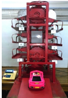
Figure 3. Loading position for car parking
