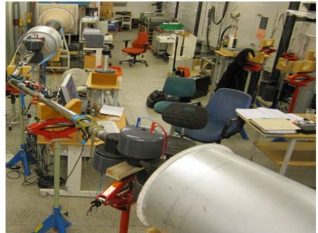
Figure 1. Measurement configuration for plane wave decomposition at MWL.(a) Constructor drawing of the test rig that is used with Case 1 (single orifice) and Case 2 (double orifices), (b) Photo for the test rig with SR is connected
