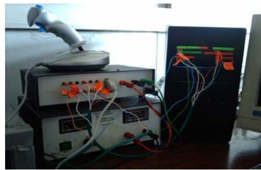
Figure 10. system controller with interfacing circuits'
