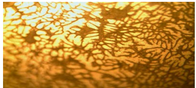
Figure 9. Microstructure of 2.5 % Cu alloy X250
