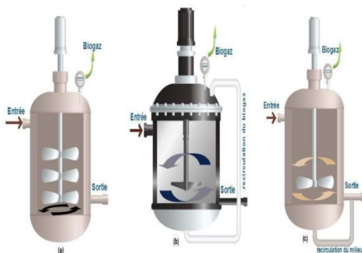
Figure 2. Examples of the perfectly mixed digester: a) mechanically by blades, b) by compression and recirculation of the biogas, c) by recirculation of the medium. [14]
