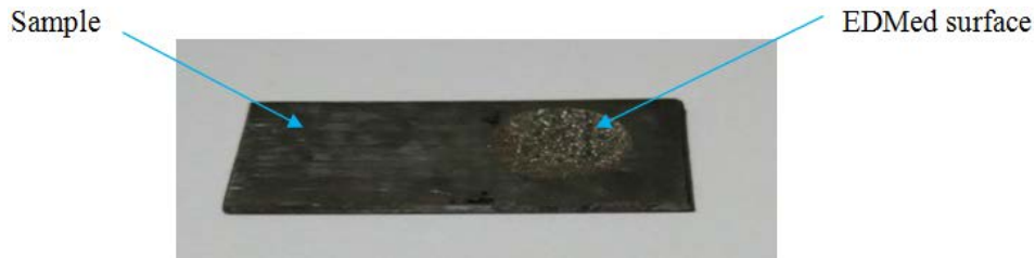
Figure 2. Edmed surface with I_p= 7.5 A, T_{on}= 15 \mu s, T_{off}= 150 \mu s, C_p= 800 MPa
