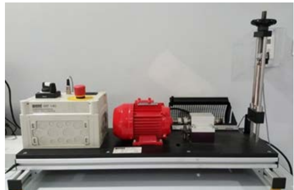
Figure 6. rotating bending testing machine (WP 140)
