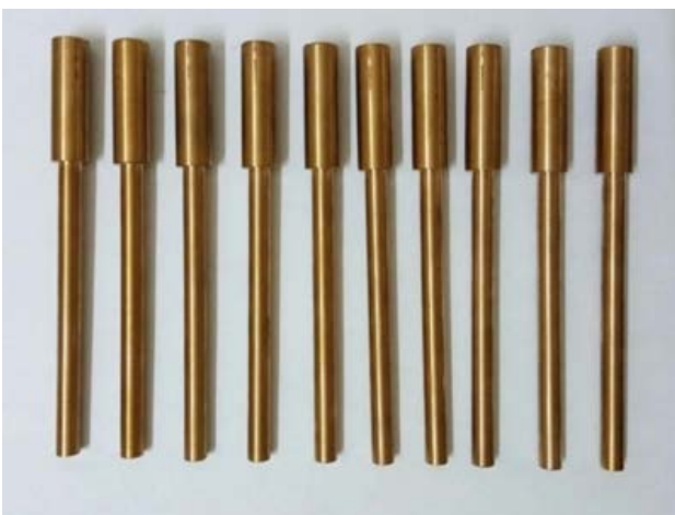
Figure 4. The specimens brass on fatigue device WP 140
