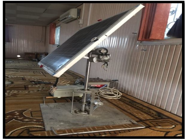
Figure 2. The proposed model for dual axis tracker
