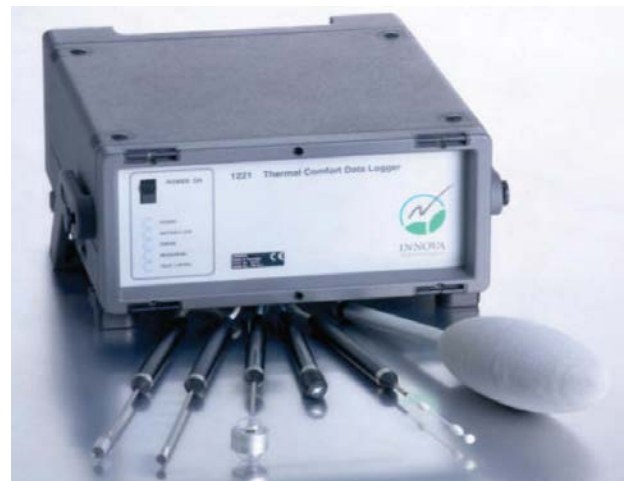
Figure 3. Thermal comfort conditions transducers used with Bruel & Kjaer Air Tech. Instruments, thermal data logger 1221, were all fitted into a trolley
