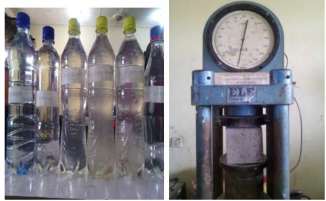
Figure 2. Water samples ready for (TDS) test (left) and Compression Testing Machine (right)
