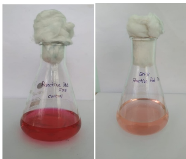
Figure 3. Biodegradation activity of S. apiospermum SKF2 against the RR 180 dye after 204hrs incubation time
