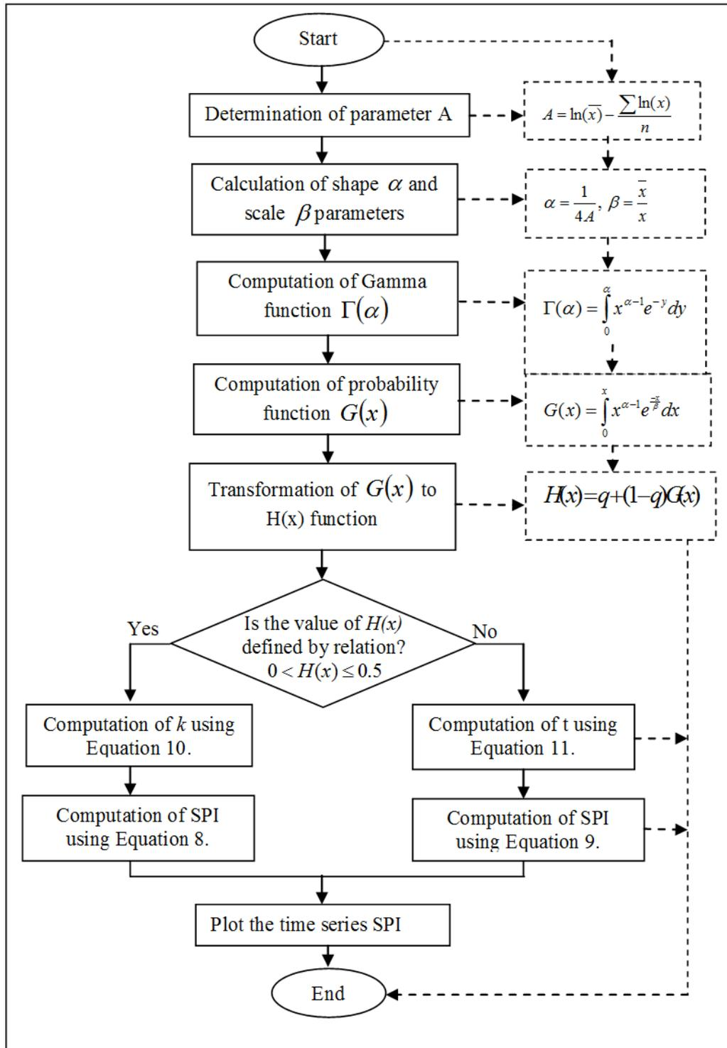
Figure 3. The flow chart of the procedure used in computation of the time series SPI
