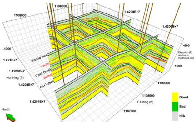
Figure 5. Zone-partitioned facies/porosity comparison model
