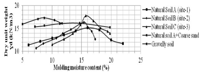
Figure 3. Compaction curve for the various natural soils
