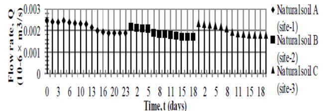
Figure 11c. Leachate flow rate against time for p = 50kPa
