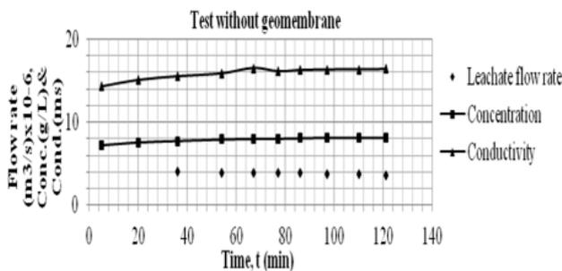
Figure 10a. Flow rate, conc. and cond. values for test without geomembrane at p = 0kPa
