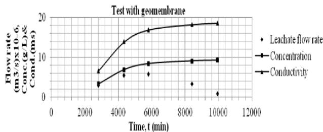
Figure 10b. Flow rate, conc. and cond. values for test with geomembrane at p = 0kPa
