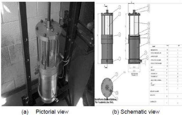
**Figure 6.** Modular consolidometer-percolation column hybrid device
