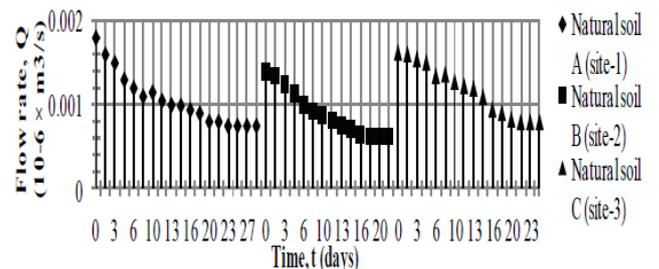
Figure 11d. Leachate flow rate against time for p = 100kPa
