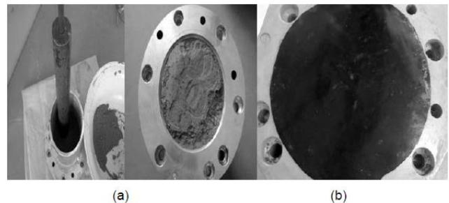
**Figure 8.** (a) Compacting the soil in layers (as CCL) in the barrier holder (b) Defected geomembrane with 5mm hole placed over CCL
