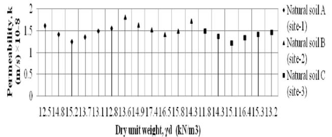
Figure 4. Permeability variation of the various soil samples
