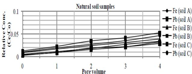
Figure 13. Relative conc. of heavy metals in effluent ( $C_o$  and  $C_e =$  initial and final conc.)
