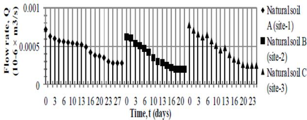
Figure 11e. Leachate flow rate against time for  $p = 150\text{kPa}$
