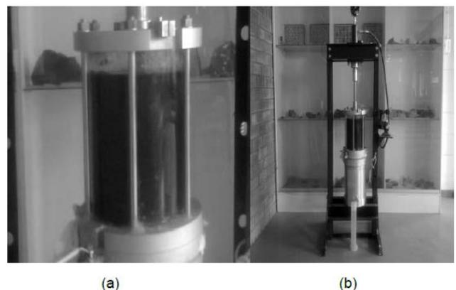
**Figure 9.** (a) Leachate in reservoir (b) Set-up under load from the hydraulic pressure system
