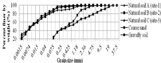
Figure 2. Grain size distribution curves for the different soils
