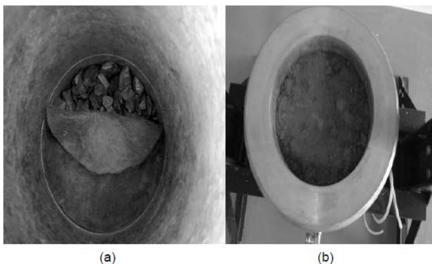
**Figure 7.** (a) Wetted geotextile on porous stone to prevent outlet clogging (b) Lightly rammed AP to simulate loosed subsoil in the chamber
