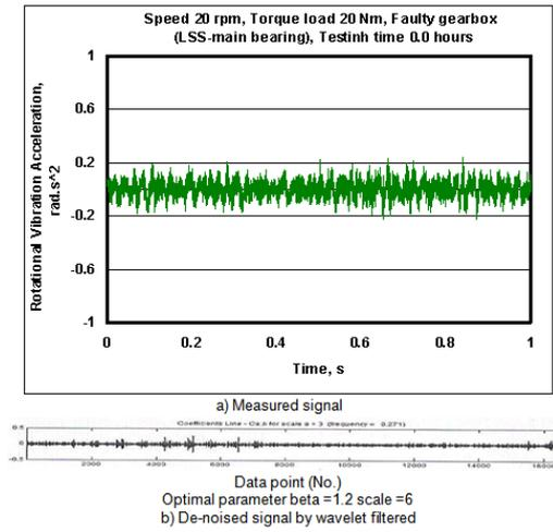
Figure 8. Vibration signal of planet gears carrier crack at 0.0 hr (20 rpm, 20 Nm)
