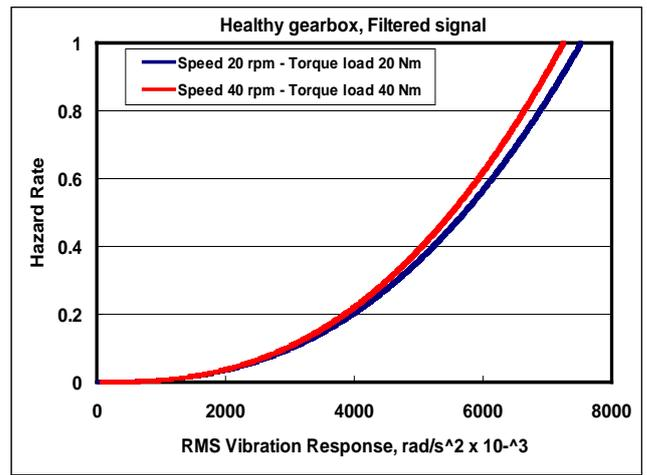
Figure 10. RMS of vibration response at failure, healthy gearbox
