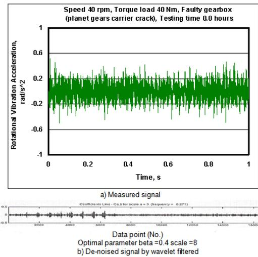
Figure 9. Vibration signal of planet gears carrier crack at 0.0 hr (40 rpm, 40 Nm)
