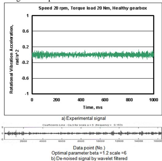
Figure 6. Vibration signal of healthy gearbox (20 rpm, 20 Nm)
