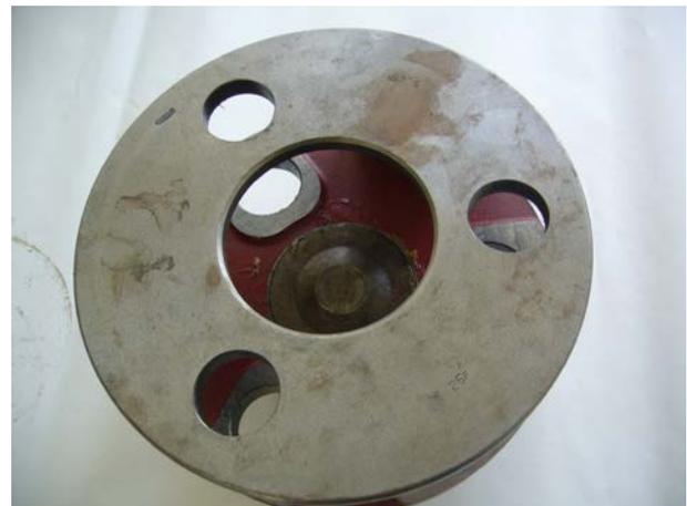
Figure 4. Planet gears carrier
