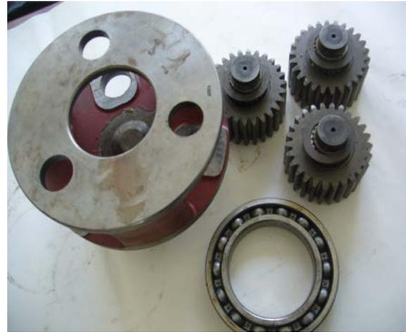
Figure 3. Planetary gearbox assembly
