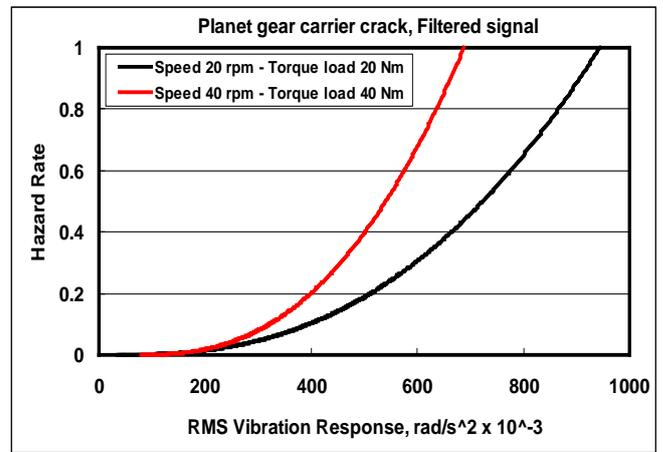
Figure 11. RMS of vibration response at failure, planet gears carrier crack
