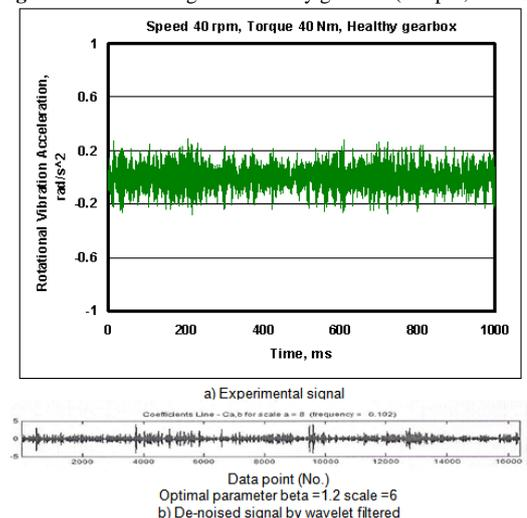
Figure 7. Vibration signal of healthy gearbox (40 rpm, 40 Nm)
