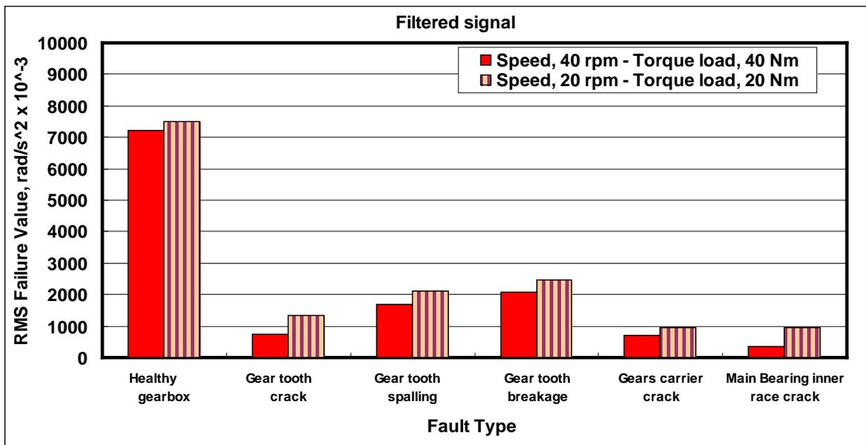
Figure 12. RMS value at failure for filtered rotational vibration acceleration signal
