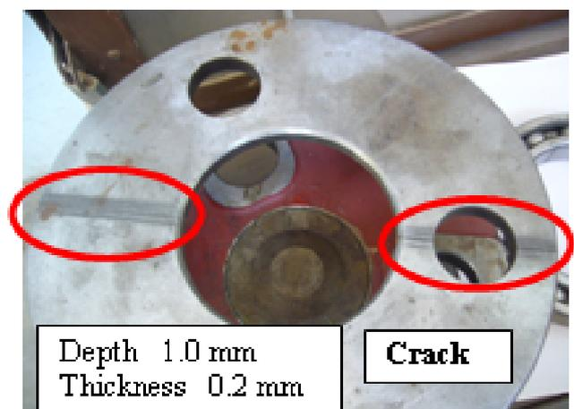
Figure 5. Planet gears carrier crack
