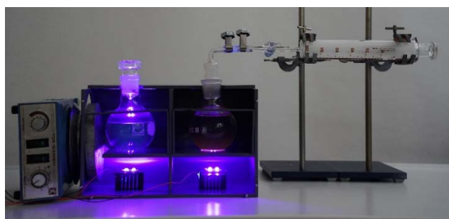
Figure 5. Experimental setup. Left: actinometry; right: hydrogen evolution.
