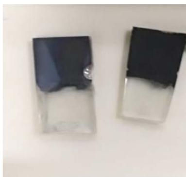
**Figure 2.** Photographic image of electrochemically deposited NiS amorphous nanostructured film
