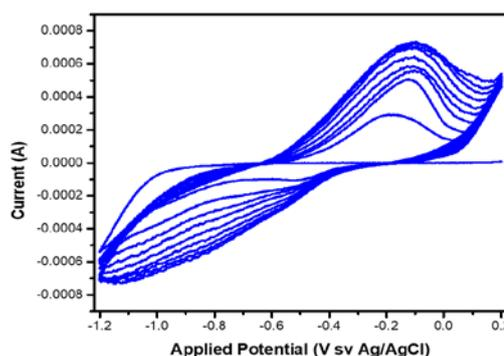
**Figure 1.** shows Cyclic voltammetry for NiS synthesis
