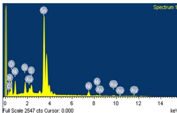
**Figure 4.** EDX analysis of NiS nanostructured film on FTO glass substrate
