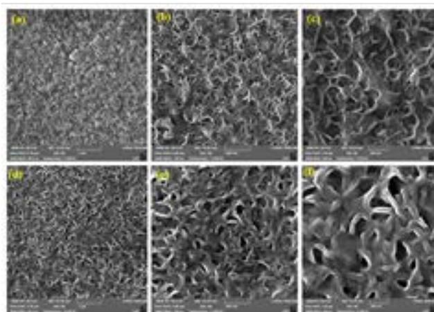
**Figure 3.** Low and High Magnification FESEM images of NiS nanostructured film grown on FTO substrate
