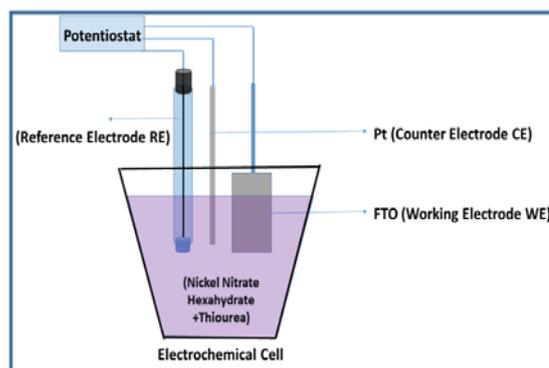
**Schematic 1.** Three electrode electrochemical deposition of NiS nanostructured amorphous films
