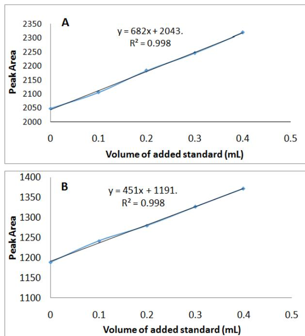
**Figure 9.** Standard addition calibration curve for Dapsone analyzed on HPLC-FLD (a) without  $\beta$ -CD, (b) after adding  $\beta$ -CD to the mobile phase. The unknown volume was 0.2 mL and the concentration of spiked Dapsone standard was 100 ppb and its volume was 0.1 mL
