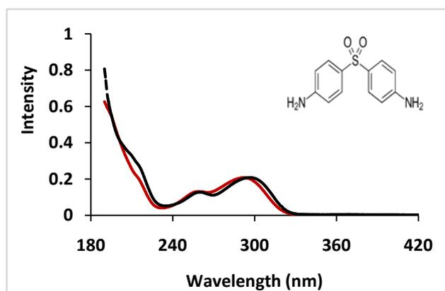
**Figure 1.** UV-Vis spectra of Dapsone in aqueous solution without adding  $\beta$ -CD (solid red line) and after adding  $\beta$ -CD (dotted black line). Dapsone structure is shown at the figure top
