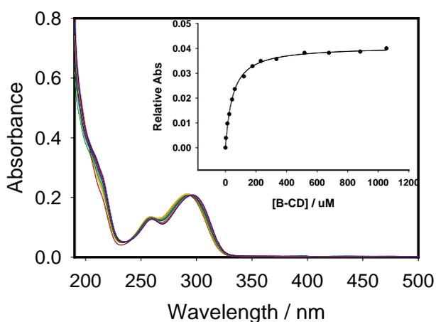
**Figure 7.** Absorption spectra between Dapsone and  $\beta$ -CD in a basic medium (pH 10). Data fit for binding constant calculation is shown in the inset ( $k = 24238.8204$ ,  $S = 4630.4750$ ,  $R^2 = 0.9964$ )
