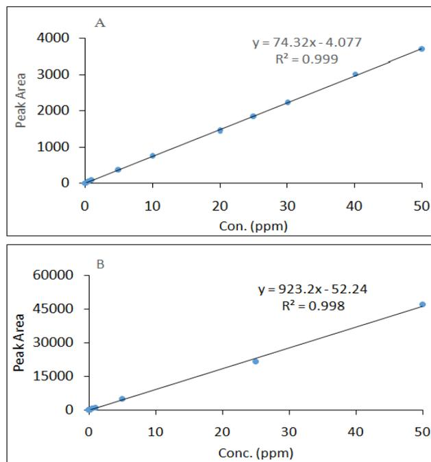
**Figure 8.** Calibration curve for Dapsone analyzed on HPLC-FLD (a) without  $\beta$ -CD, (b) after adding  $\beta$ -CD to the mobile phase
