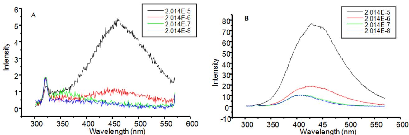
Figure 2. Fluorescence spectra of Dapsone at different concentrations ( $2.014 \times 10^{-5}$  -  $2.014 \times 10^{-8}$  M) (A) without and (B) with  $\beta$ -CD
