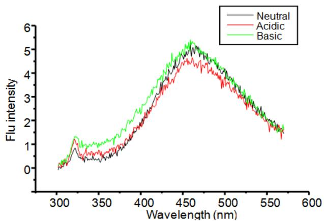
**Figure 4.** Fluorescence spectra of Dapsone drug in acidic, neutral and basic solutions ( $[Dapsone] = 2.0 \times 10^{-6} M$ )
