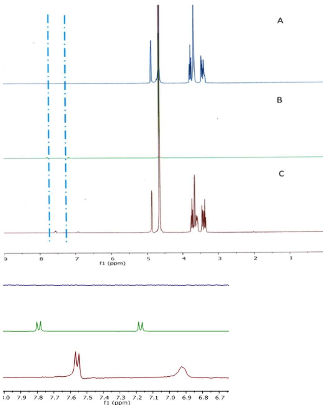
**Figure 6.**  $^1\text{H-NMR}$  spectra for (A) 2.93 mM  $\beta$ -CD, (B) 1.54 mM Dapsone and (C) 1.54 mM Dapsone- and 3.23 mM  $\beta$ -CD mixture (top figure).  $\text{D}_2\text{O}$  was used as solvent in all the experiments. A close up to the NMR signal (6.6-8.0 ppm) is shown in the bottom figure
