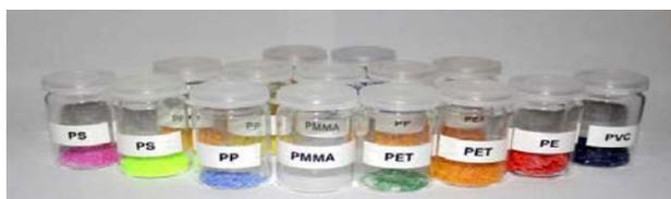
**Figure 1.** Snap top vials with micro-plastic samples for the model experiment of the sediment analysis. These were made as various everyday objects, which can still be assigned with the help of the colours even after the analysis
