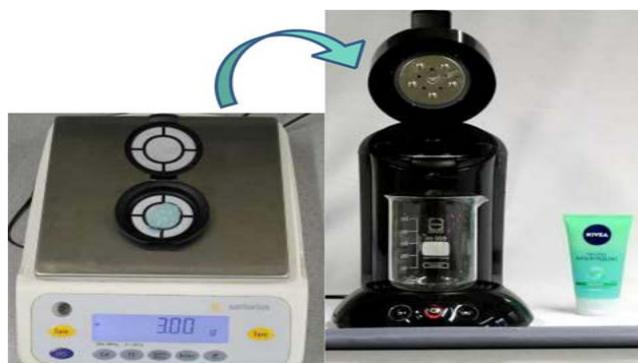
**Figure 5.** Weigh out 3 grams of cosmetic peeling in a permanent coffee filter (left) and transfer to the coffee pad machine (right). Then the sample is rinsed up to seven times until no more gel-like components of the peeling are present
