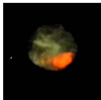
Figure 10. Picture from the video recording of triboluminescence of  $[\text{Eu}(\text{DBM})_4\text{TEA}]$
