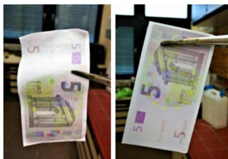
**Figure 7.** Hydrophobic effect of sodium stearate. Left: banknote glued with sodium stearate, right: non-glued banknote, both soaked in water
