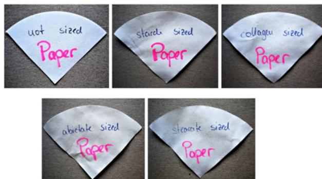
Figure 1. Sizing effect of the tested sizing agents
