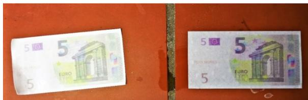
**Figure 8.** Opacity of an impregnated (left) and non-impregnated banknote (right)
