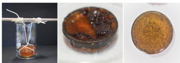
Figure 6. Fabrication of polymer coated with silver nanoparticles (left, center); silver nanocomposite with visible inclusions (right)
