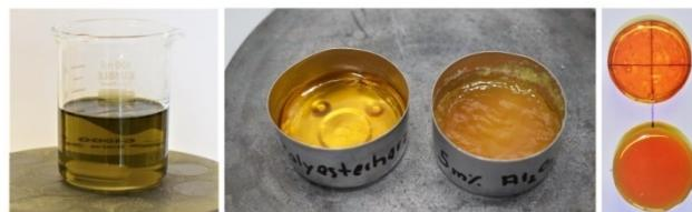
Figure 3. Preparation of the basic mixture (left); hardening of polymer and nanocomposite in tea light shells (center); transparent polymer and opaque nanocomposite (right)
