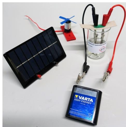
Figure 6. Generation of the fuel via electrolysis with a battery
