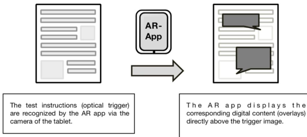
Figure 1. Operating principle of an AR worksheet
