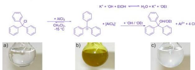
**Figure 5.** Reaction of chlorotriphenylmethane with aluminum(III) chloride and potassium hydroxide in dichloromethane. a) shows the solution of chlorotriphenylmethane in dichloromethane, b) the solution 2 min after the addition of aluminum(III)chloride and c) the solution after the addition of 3 mL potassium hydroxide in ethanol
