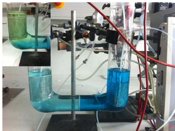
**Figure 14.** Simple setup that shows the color change of the anode region after charging and discharging
