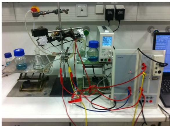
**Figure 11.** Experimental setup VRFB. From left to right: Pumps, reservoirs for the vanadium solutions, cell (between the pumps), power supply for charging, motor and data logging
