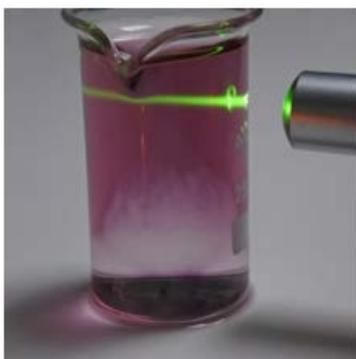
**Figure 5.** Detection of gold-nanoparticles by Faraday-Tyndall-effect
