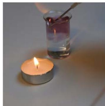
Figure 4. Reducing of gold(III)chloride-solution with burning hydrogen. The candle-light was used to ignite the hydrogen.
