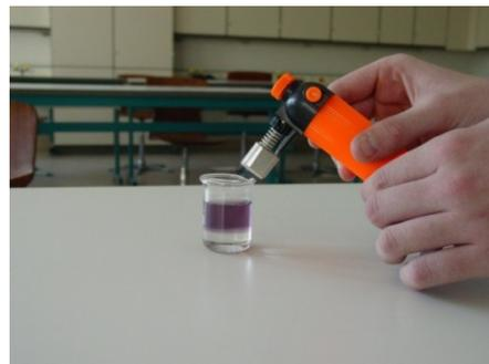
Figure 3. Reducing of gold(III)-ions with a propane burner
