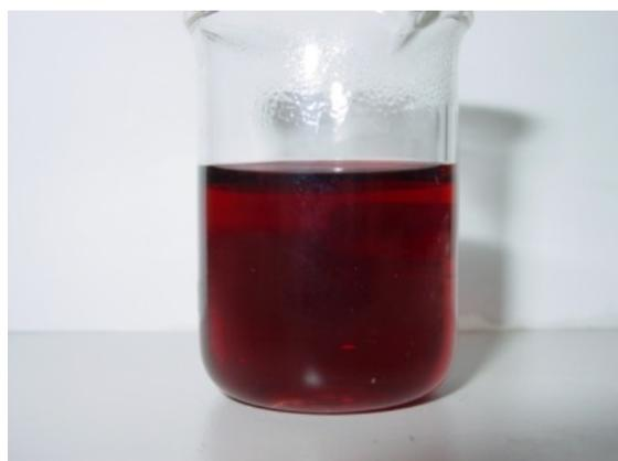
**Figure 10.** Gold nano colloids prepared from  $10^{-3}$  M  $\text{HAuCl}_4 \cdot 3 \text{H}_2\text{O}$  and dry red wine
