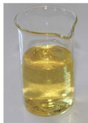
**Figure 12.** Silver-Nanoparticles from Creighton-method
