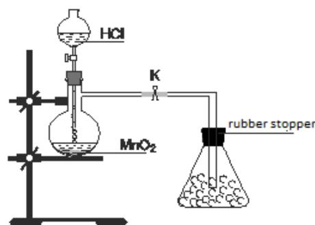
Figure 2. The apparatus was used to prepare chlorine gas
