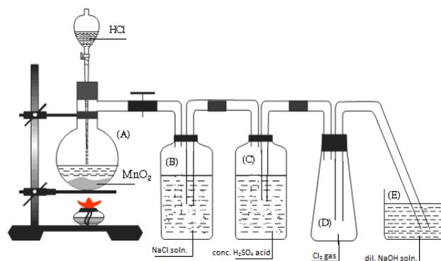
Figure 3. The apparatus was used to prepare and collect chlorine gas
