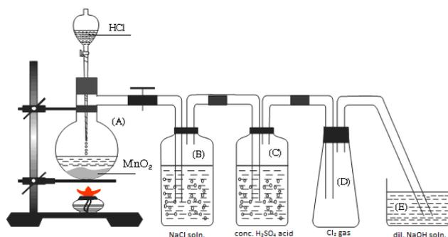
Figure 4. The apparatus was used to prepare and collect chlorine gas
