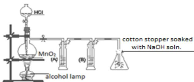
Figure 1. Collecting pure chlorine gas
