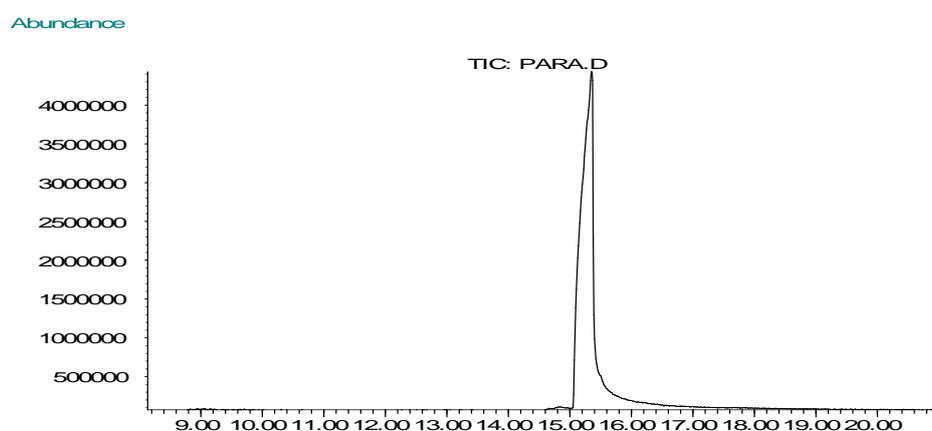
Figure 9a. Part of the GC-MSD of paracetamol (100  $\mu\text{mol/L}$ , injection 1  $\mu\text{L}$ ).GC (Hewlett-Packard, 5890 SII), MS (Hewlett-Packard 5972) with capillary column (RTX-35 Restek);helium as carrier gas. Temperature profile: 50°C (1 min isotherm) to 280°C (temperature rate 15°C/min), 280°C (5 min isotherm); Autosampler (Hewlett-Packard, 7673)
