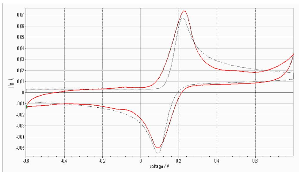
Figure 3. Experimental (red) and fitted (black) CV curves of paracetamol with CNT-GNP SPE
