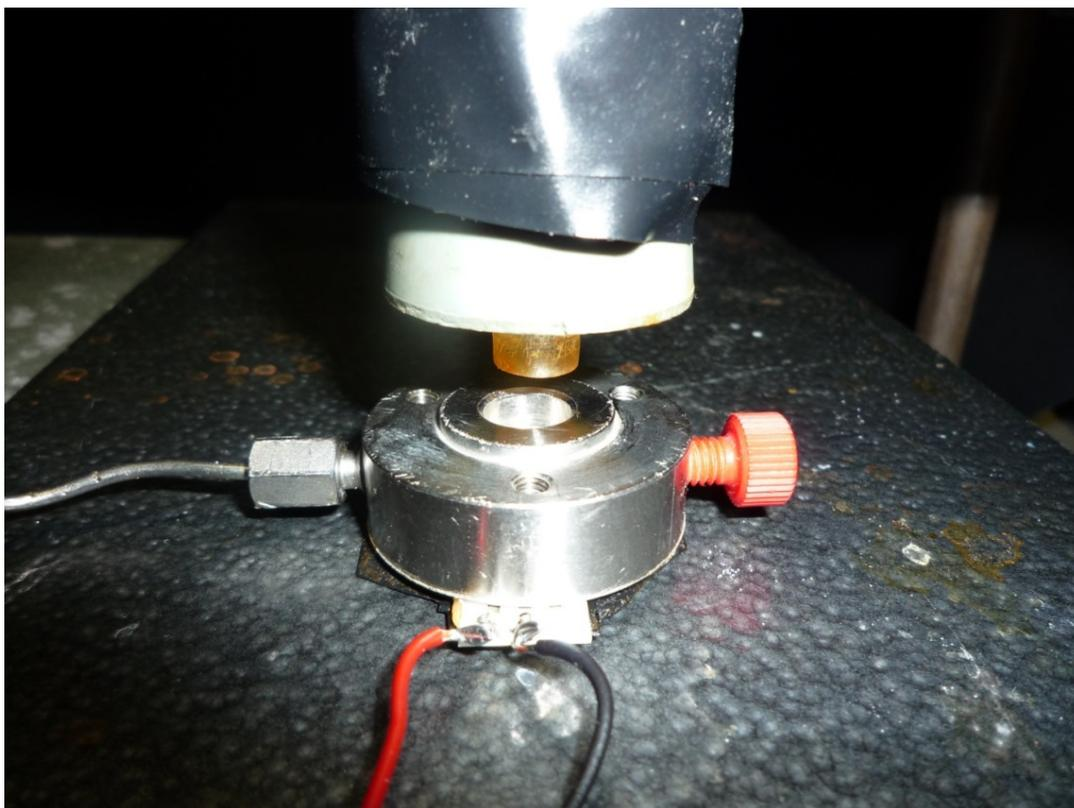
**Figure 7.** An ECL cell for ECL. The SPE is fixed below the cell. Volume is about 80  $\mu\text{L}$ . The fiber guides the ECL into the photomultiplier and is inserted into the hole of the cell
