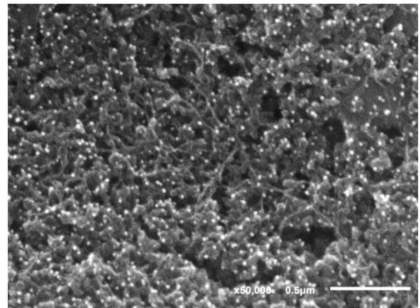
Figure 2. Electron microscope image of the CNT-GNP SPE. The white dots are the Au nanoparticles that coat the CNT surface
