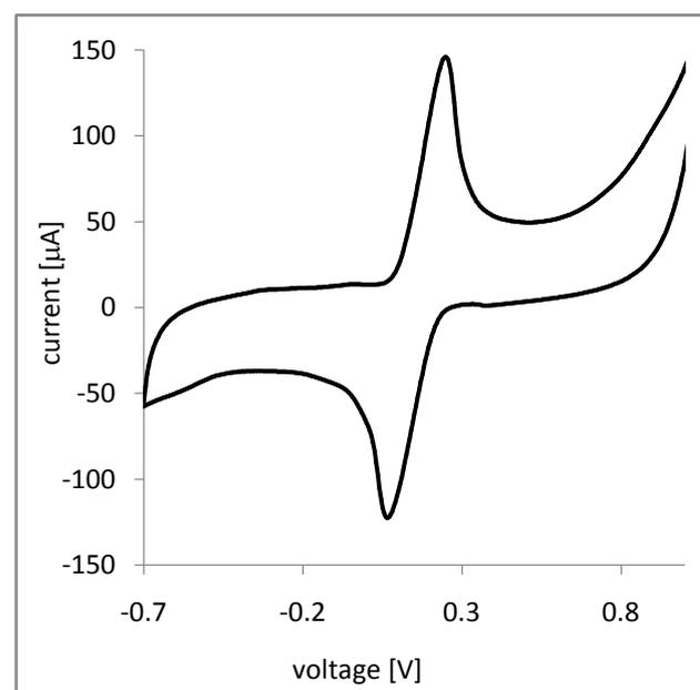
**Figure 1a.** CV of paracetamol (1 mmol, pH 8) with different SPEs (Figures with the same ordinate).SPE: CNT-GNP
