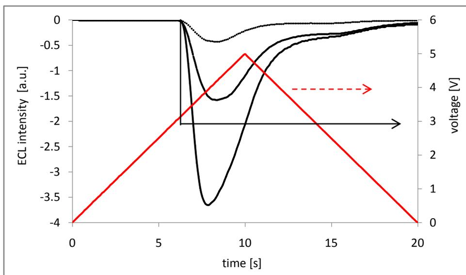
**Figure 8a.** ECL of  $[\text{Ru}(\text{bpy})_3]^{2+}$  - prolinealone (solid line) and with paracetamol (5  $\mu\text{mol/L}$  (dashed line) and 10  $\mu\text{mol/L}$  (dotted line). The red curve represents the applied angular voltage (5V in 10 s)
