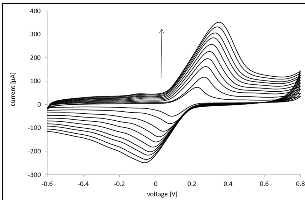
**Figure 4.** CV of paracetamol with a CNT-GNPSPE. Scan rate: 10–100 mV/s. Slower scan rates yield lower currents. The arrow indicates increasing scan rate
