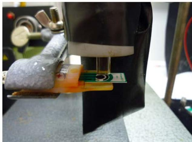
**Figure 2.** Experimental setup. Top: From left to right: programmable pulse-generator (Power Cassy), data acquisition system (Sensor Cassy), photomultiplier tube with glass fiber above the SPE. Bottom: Part of photo above with clearly seen SPE and glass fiber
