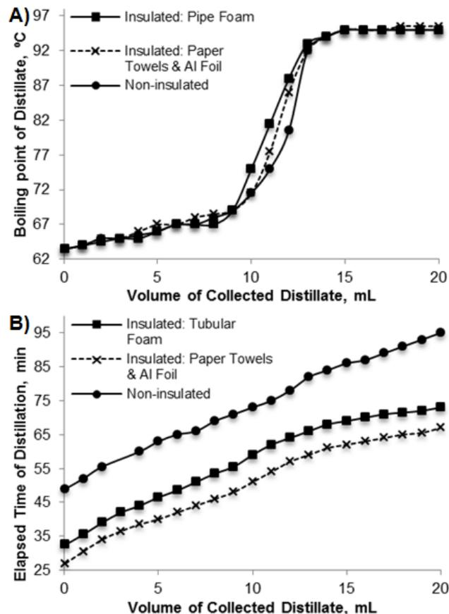
**Figure 3.** Data for the separation of a 50% (v/v) methanol and 1-propanol mixture under similar conditions with a Vigreux fractionating column that was either non-insulated or insulated with either tubular polyethylene foam or paper towels and aluminum foil, respectively. A) Fractional distillation plots of boiling point versus volume of collected distillate. B) Plots of elapsed time of distillation versus volume of collected distillate
