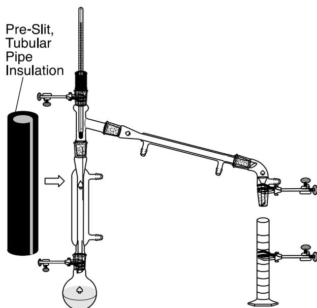
**Figure 1.** Schematic for employing pre-slit, tubular pipe insulation with a fractional distillation apparatus
