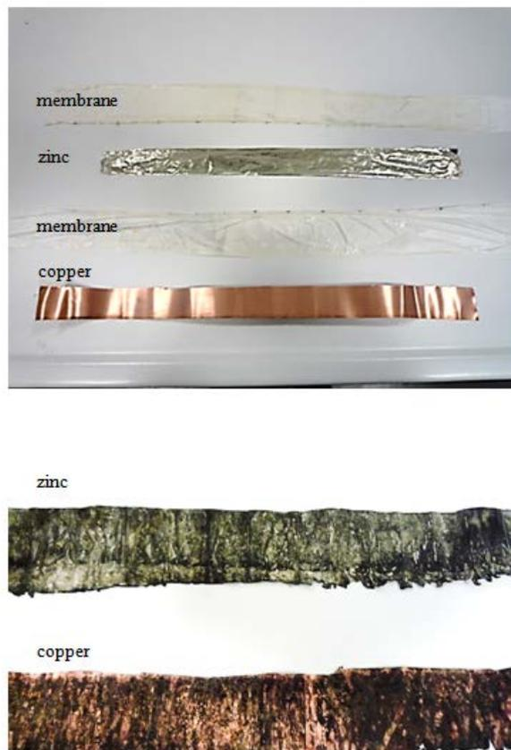
**Figure 13.** Photos of the used copper and zinc sheet. Top: before, bottom: after use as electrodes in the Cu-Zn battery. On top: white: the separators. The materials were wound as a sandwich: Cu - separator - Zn - separator. Metal loops at the end of the two metals were connected with alligator clips
