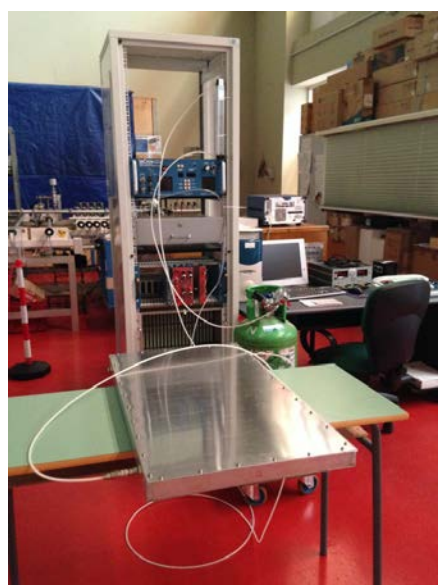
Figure 14. The MRPC is ready for flushing gas
