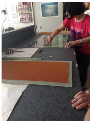
Figure 4. Preparation of the honeycomb panels
