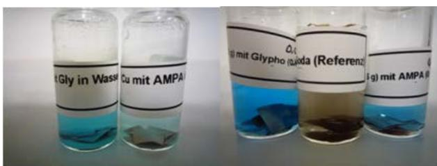
**Figure 1.** left: Copper sheets in water with glyphosate (left) and with AMPA (right); Right: Copper sheets in sodium carbonate with glyphosate (left), with AMPA (right), and without glyphosate or AMPA (middle)
