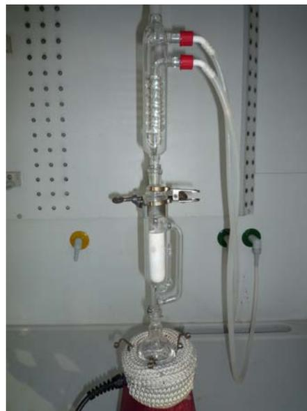
**Figure 12.** Extraction equipment: heater, flask, Soxhlet with extraction thimble containing glyphosate and soil, and the reflux cooler.
