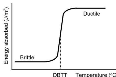
**Figure 5.** Ductile-to-brittle transition behavior in BCC metals
