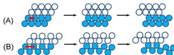
**Figure 4.** Shear planes in (A) closely packed FCC and (B) loosely packed BCC structures during applied stress. The length of the “slip distance” is represented by the red arrow
