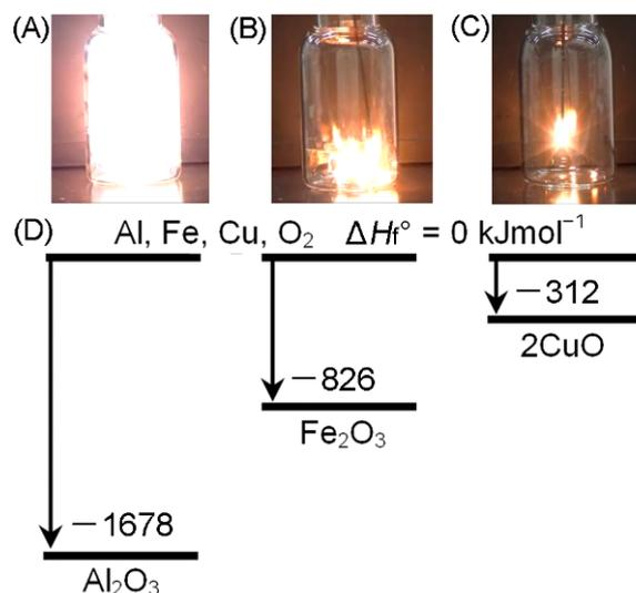
**Figure 1.** Metal burning experiments in an oxygen atmosphere: (A) aluminum foil, (B) steel wool, (C) copper foil, and (D) heats of formation ( $\Delta H_f^\circ$  ( $\text{kJ mol}^{-1}$ )) of the corresponding oxides [11]
