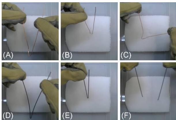
**Figure 2.** Cooling of metal wires on dry ice followed by straightening. Copper wire (A) before cooling, (B) pressed against dry ice, and (C) straightening after cooling. Steel wire (D) before cooling, (E) pressed against dry ice, and (F) breaking upon straightening
