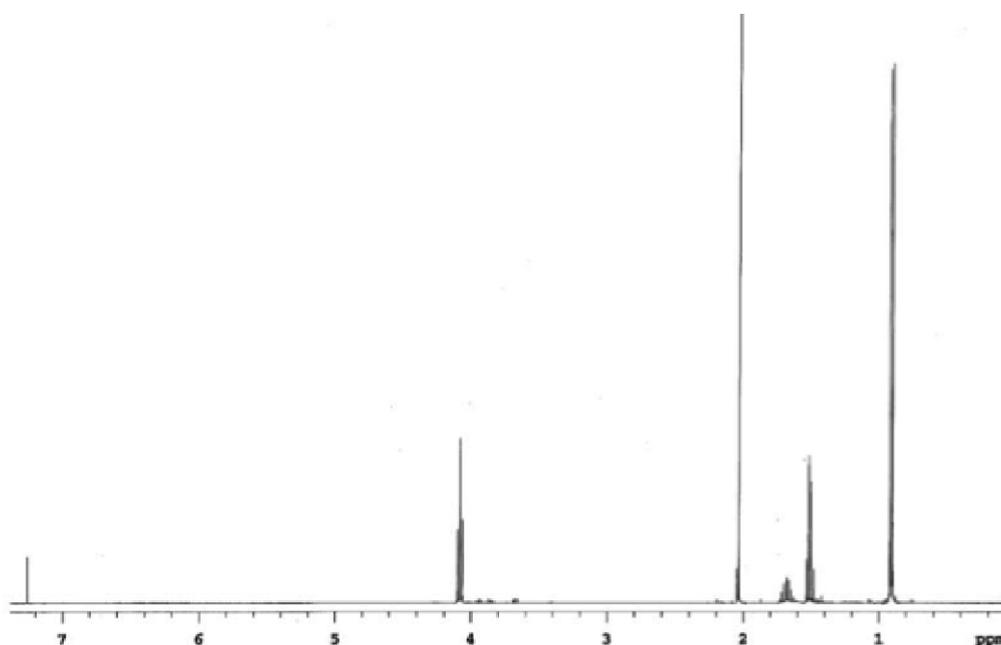
**Figure 2.** Sample <sup>1</sup>H NMR obtained by the laboratory students. Pictured is Unknown Product 4, or isoamyl acetate. The <sup>1</sup>H NMR is either obtained by the student or provided in the manual. Determining product structure from the <sup>1</sup>H NMR allows the student to accurately identify what alcohol was reacted with the acetic acid
