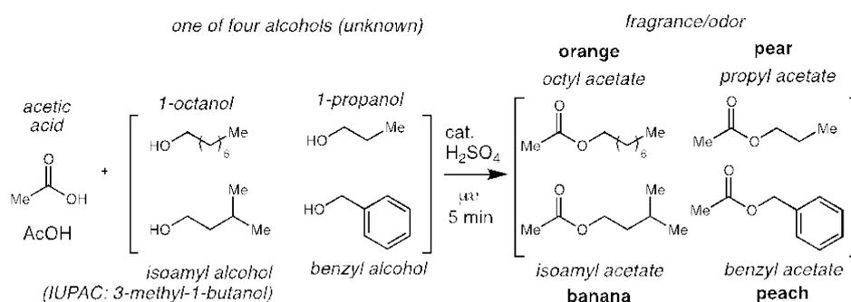
Figure 1. Protocol for the microwave esterification including the alcohols used as unknowns and the corresponding synthesized esters. Each produced ester displays a distinct fruity smell; isoamyl acetate-banana, propyl acetate-pear, benzyl acetate-peach, and octyl acetate-orange
