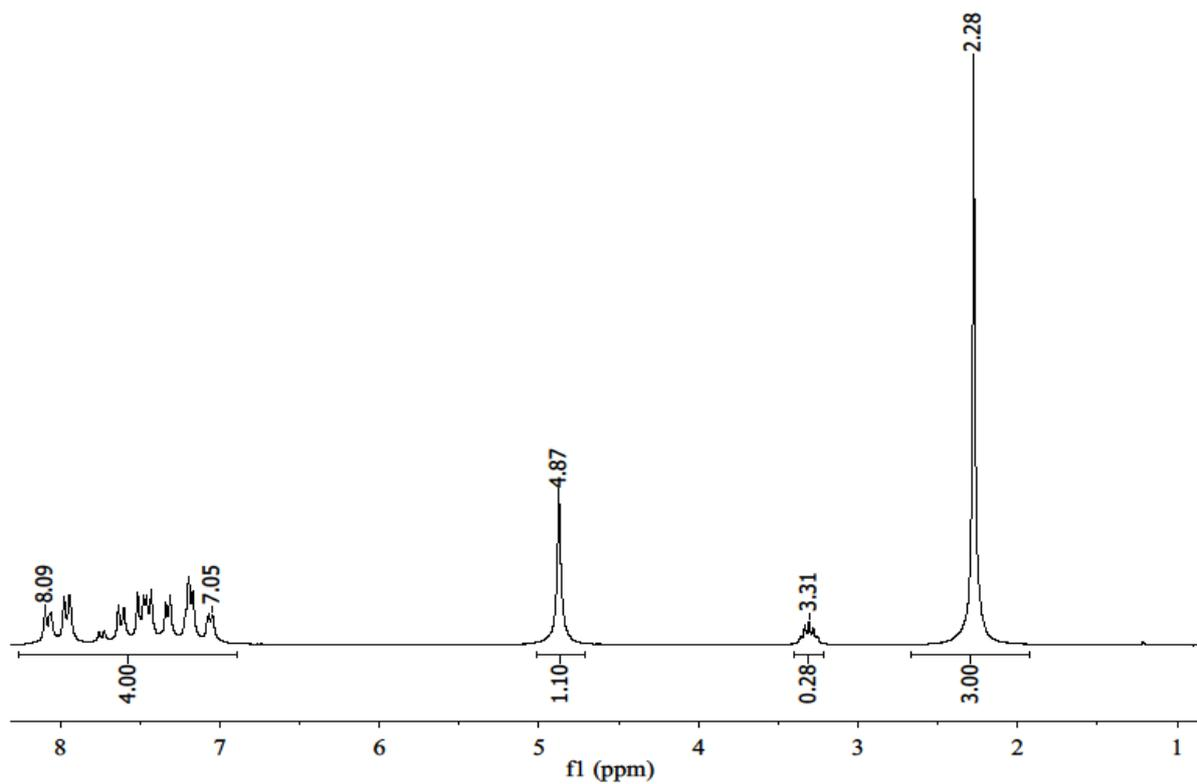
**Figure S7.** The  $^1\text{H}$ -NMR spectrum of the final product, acetylsalicylic acid in *d*-methanol with 0.03% TMS
