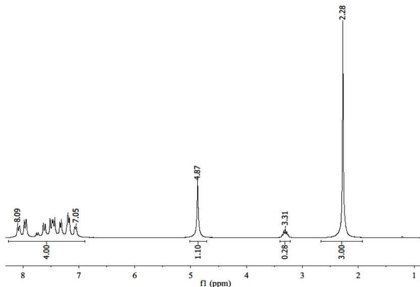
**Figure 4.** The  $^1\text{H-NMR}$  spectrum of the final product of ASA showing the resonances with integrals that were used for quantification of the yield. The integral of the methyl resonance (2.88 ppm) was set to 3.00 and the resonances in the aromatic chemical shift region showed 4.00. In addition, the area of the methyl group in methanol (3.31 ppm, 0.28) and the water signal (4.87 ppm, 1.10) are shown
