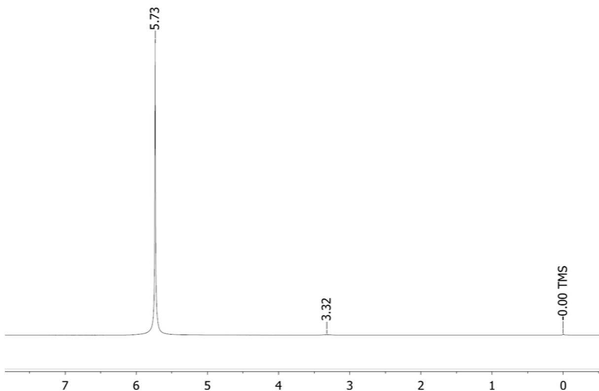
**Figure S5.** The <sup>1</sup>H-NMR spectra of phosphoric acid (85%) in *d*-methanol with 0.03% TMS. No impurities were found
