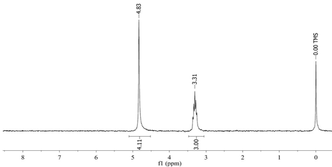
Figure S2. The  $^1\text{H-NMR}$  spectra of *d*-methanol with 0.03% TMS
