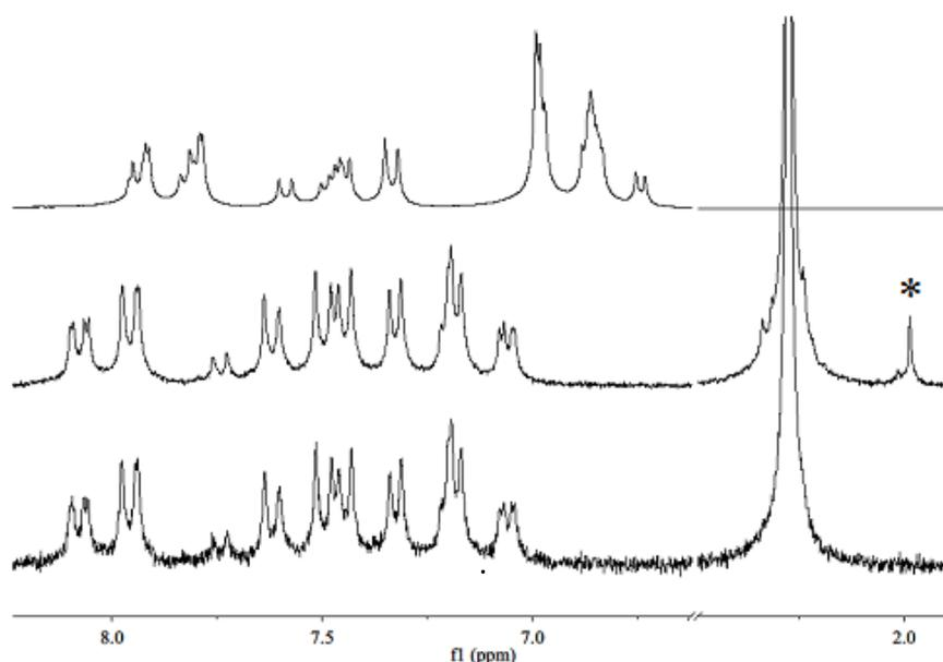
**Figure 3.** Spectrum top to bottom, show the  $^1\text{H-NMR}$  spectra of SA (top), the crude product ASA (middle) and the final product, ASA (bottom). The cutout of the  $^1\text{H-NMR}$  spectra includes the regions where we find the methyl group (1.6-3.00 ppm) and the aromatic region (6.6-8.5 ppm)
