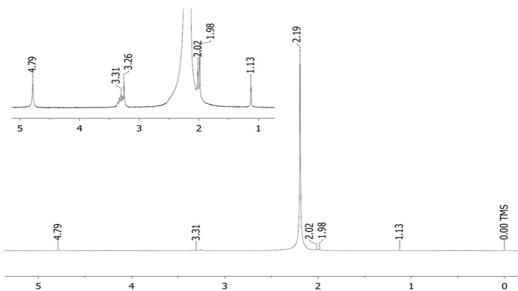
Figure S4. The  $^1\text{H-NMR}$  spectra of acetic acid anhydride in *d*-methanol with 0.03 % TMS. The cutout spectra show the area of 1-5 ppm and includes resonances from impurities, solvent, and satellites
