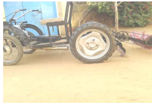
Plate 1. Side view of the machine (diggers and rotating cylinder at raised position)
