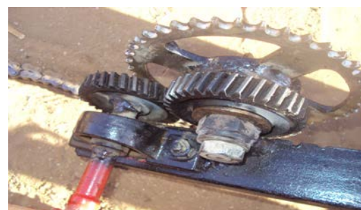
Plate 3. Second phase motion transmission (from middle gear to rotating cylinder)
